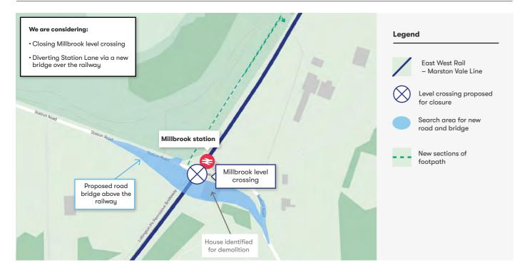
Figure: Option 1: new road bridge south west of Millbrook station
