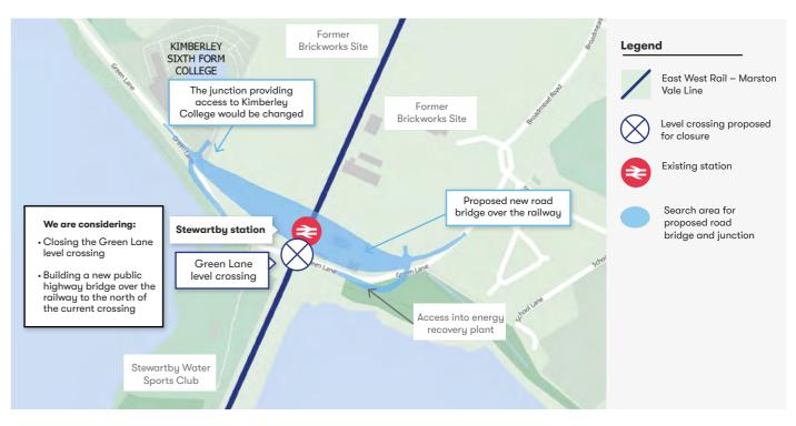
Figure: Option 1: new bridge to the north of the relocated Stewartby station
