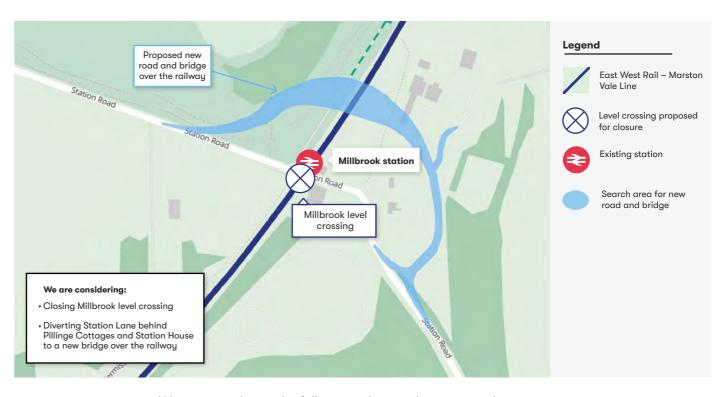
Figure: Option 3: new road bridge to the north east of Millbrook station
